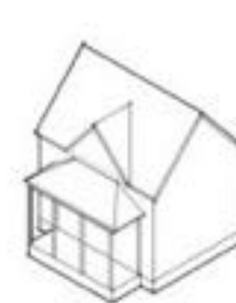
BROAD ROOF W/GABLE FRONT TYPICALLY 3 BAY 28' - 34' WIDE
