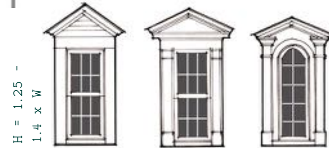
Dormers only have one window and are proportioned similarly to the windows in the
